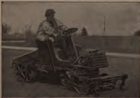
The Lawn Mower at Work, Showing the Seat and Cover, and the Convenient Control
